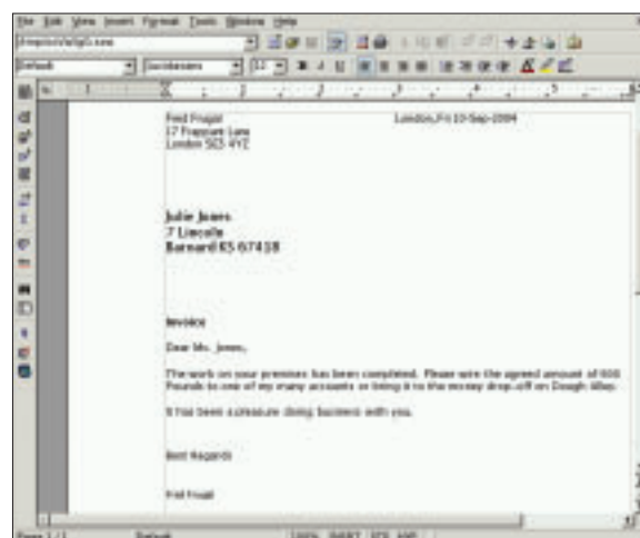
Figure 3: The document to be printed, after Mailit has completed its work on the template (Figure 1): subject line and body text from the plain text in Figure 2 have been inserted, as well as the addressee and the date.
