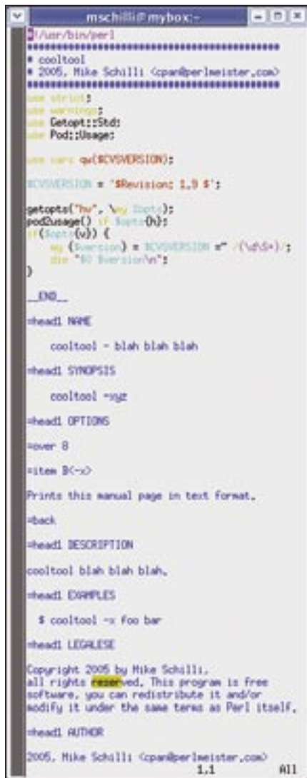
Figure 5: A template for a new script called cooltool , created by the tmpl script.
