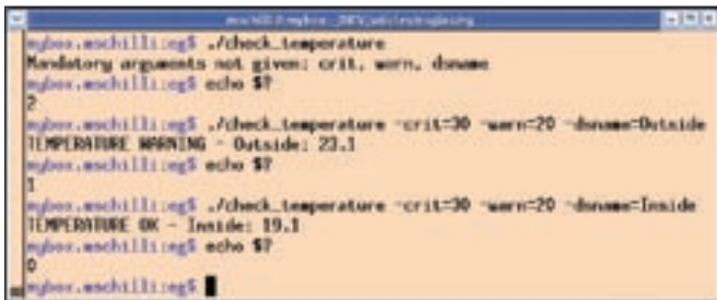
Figure 5: Output and exit values from the temperature plugin with various command line parameters.
