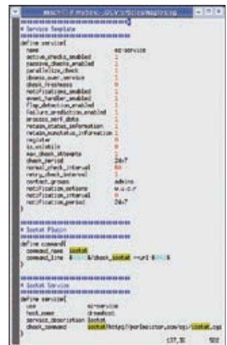
Figure 4: The Nagios configuration for the new check_temperature plugin.
