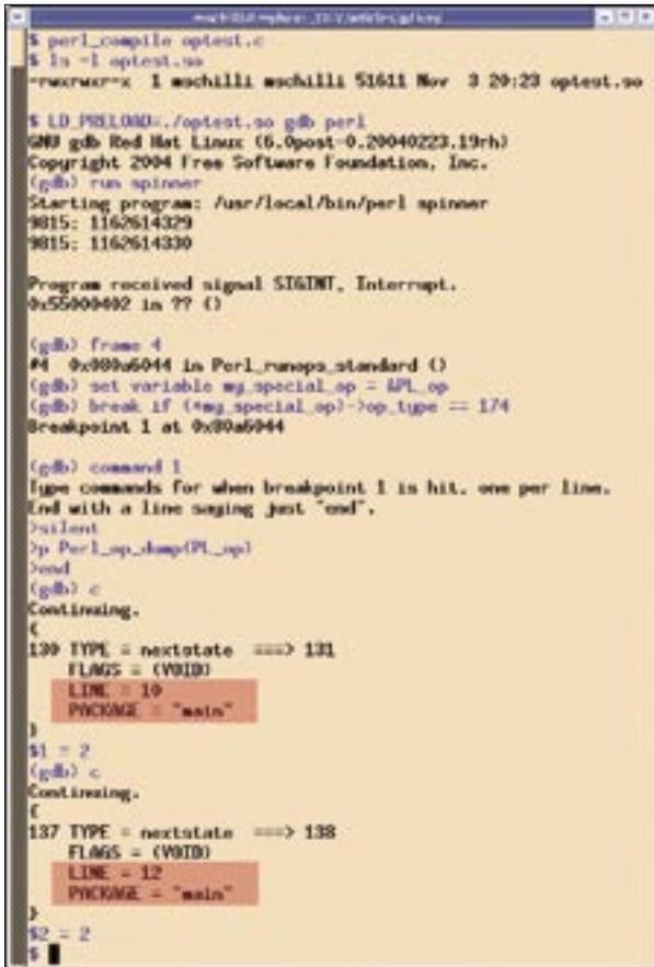
Figure 3: Discovering which line of an active Perl script is currently being processed, without debug information.
