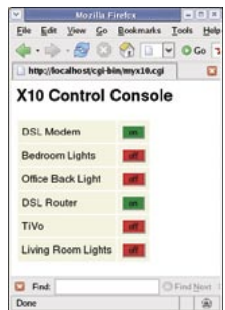
Figure 2: The interactive browser application controls multiple X10 devices at the push of a button via an intuitive GUI.
