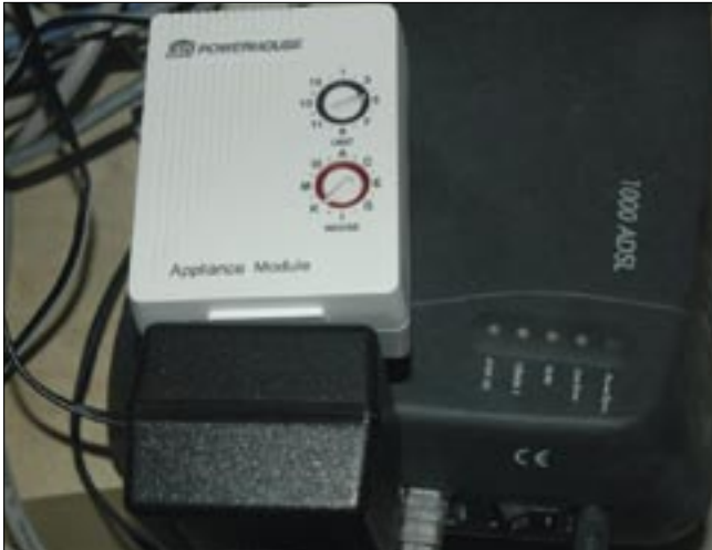
Figure 1: The DSL modem's power cord is plugged into an X10 receiver, allowing me to switch it on and off remotely, if necessary.
