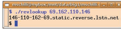
Figure 2: A reverse DNS lookup often reveals the domain associated with the IP address.
