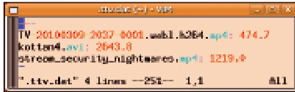
Figure 3: The script uses a YAML file ( ~/ttv.dat ) to store the elapsed viewing time for a video. Videos not stored here are played right from the beginning when the user selects them.
