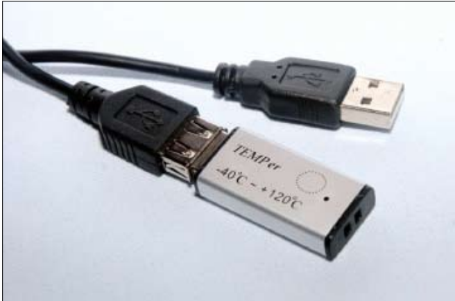
Figure 1: The affordable TEMPer USB Thermometer sensor.
