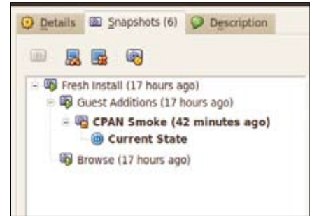
Figure 10: A new CPAN Smoke snapshot, derived from a vanilla Ubuntu install with the Guest Additions, plus a configured and ready-to-run CPAN shell.
