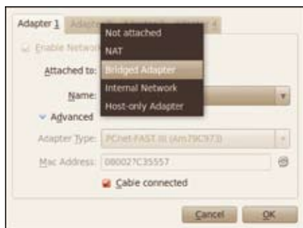
Figure 6: The Bridged Adapter in the network dialog supports bidirectional communications between the virtual machine and the rest of the world.
